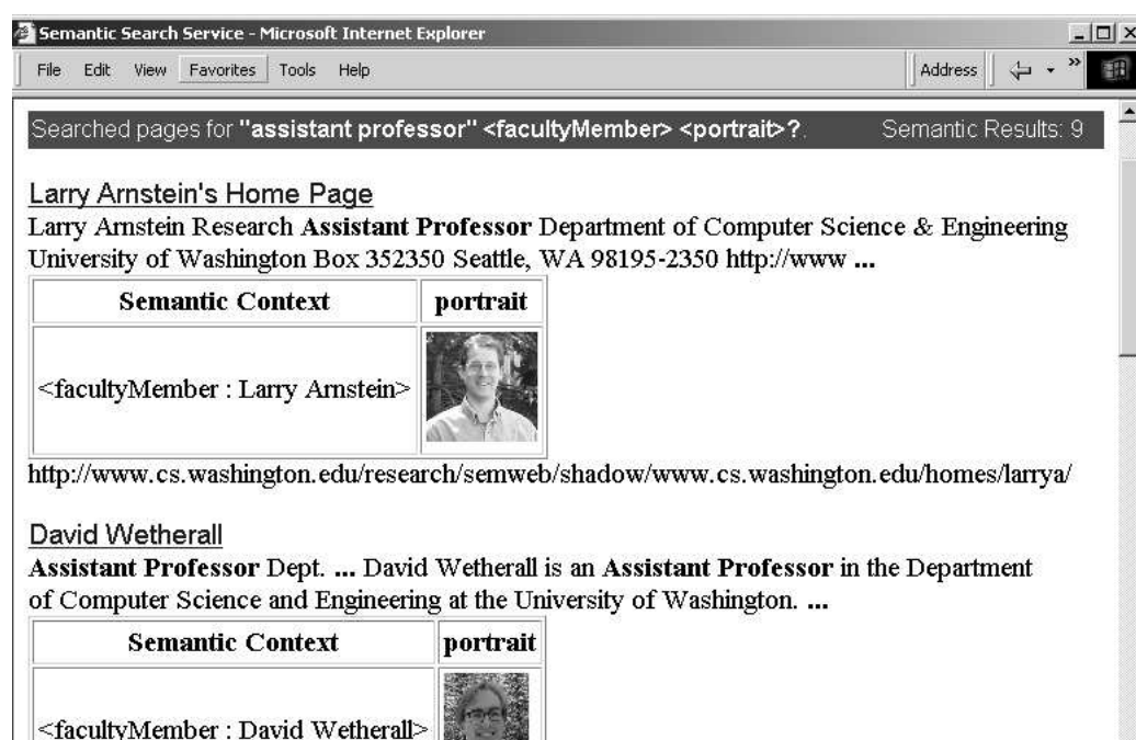
Figure 3.6: The semantic search results page. The page reproduces the original query and reports the number of results returned at the top. Matching pages contain the phrase “assistant professor” and the properties <facultyMember> and <portrait> . The ? in the query instructs the service to extract the <portrait> from each matching page.
